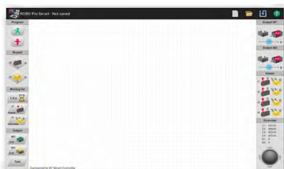
Tap on the display text that appears. The tablet or smartphone is then coupled to the controller. Successful coupling can be recognized by the fact that all commands now appear on the working display. Now the blue LED also illuminates continuously.
