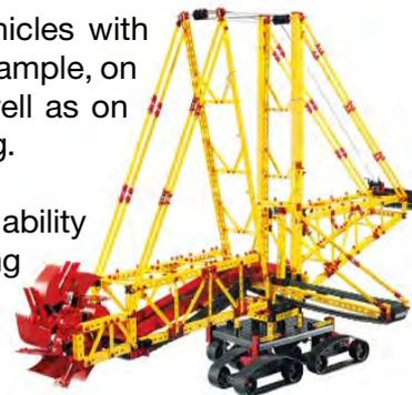
They are steered by allowing the tracks to run at different speeds on each side. For example, to turn to the left, it is necessary for the track on the right side to move faster than the track on the left. They can even turn in place by stopping one track completely.
